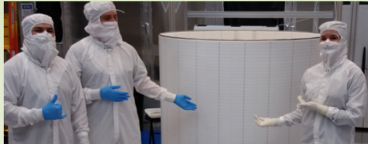
TPC Field shaping rings stacked at SURF
