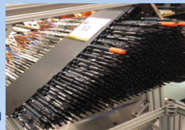
Final production petal, loaded with fiber positioners
