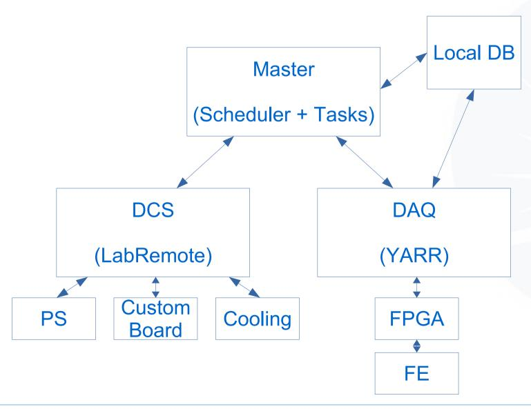
Viewer • With the local DB, extras such as viewers (web / grafana or otherwise) can be used. Local DB Master (Scheduler + Tasks) **DCS DAQ** (LabRemote) (YARR) Custom PS Cooling **FPGA** Board FΕ
