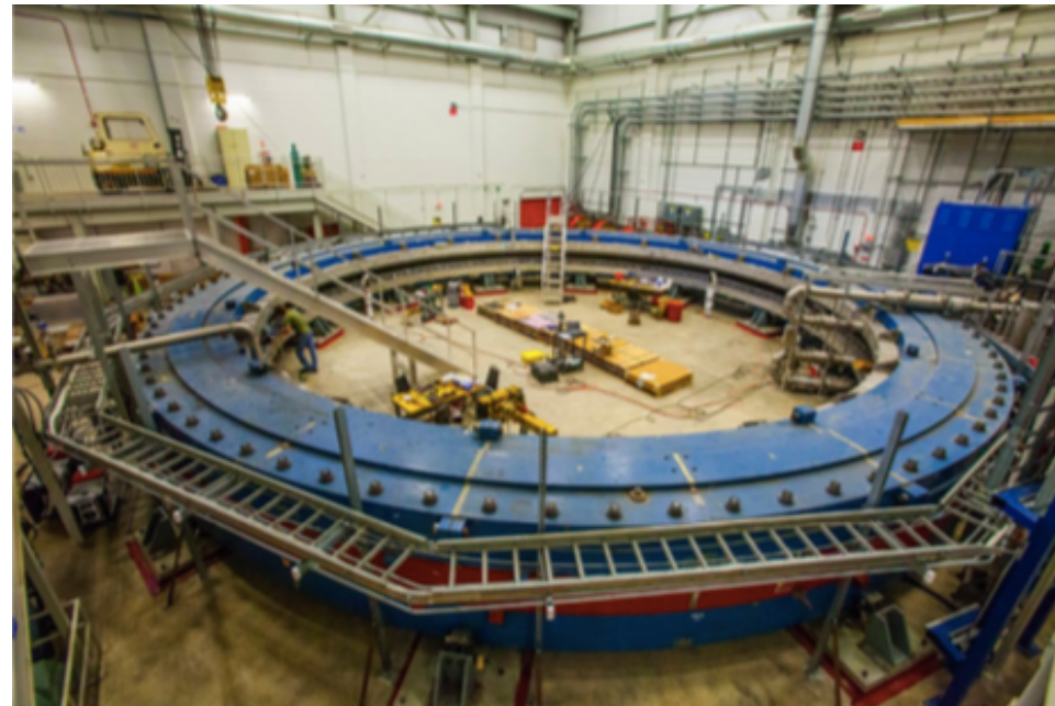
The muon storage ring at currently at Fermilab. It's essentially a large circular dipole magnet outside lead-fluoride electromagnetic calorimeters.
