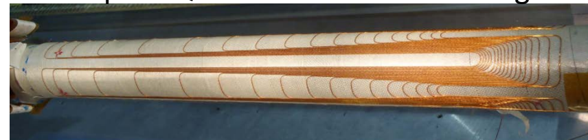
S.C. coil for QC1E magnet
