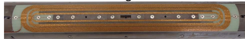
S.C. coil for QC1E magnet
