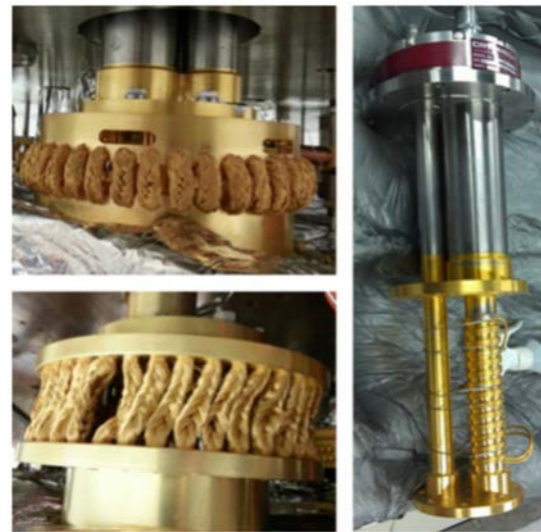
above: CUORE pulse tube and copper thermalization at 40K and 4K stages.
