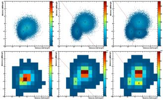
Figure 8: Energy deposit of neutral pions and their decay products in the calorimeter with different cluster shapes with fine granularity (upper row) and how they would look with the approximate resolution of the EMCal (lower row). The red dashed lines indicate the approximate splitting done by the v2-clusterizer, while the v1 clusterizer would see them as one single cluster with different number of local maxima.
