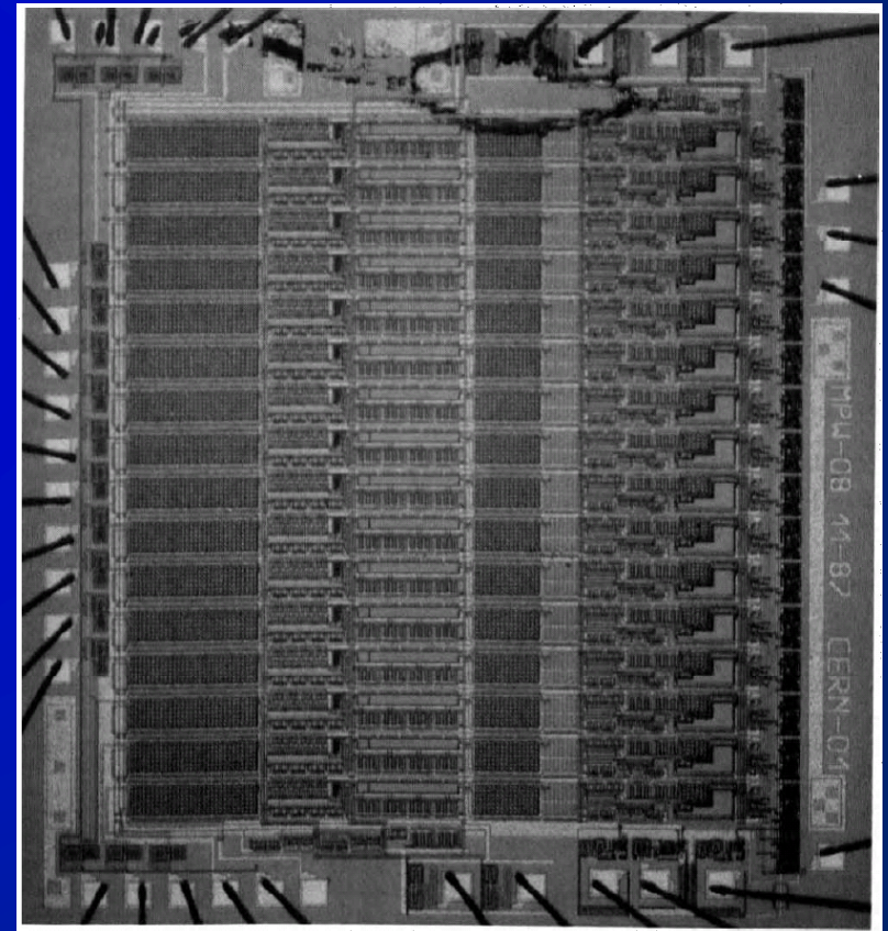
Fig. 7. Picture of the 16-channel AMPLX chip. The size is 4.1 × 4 mm 2 .
