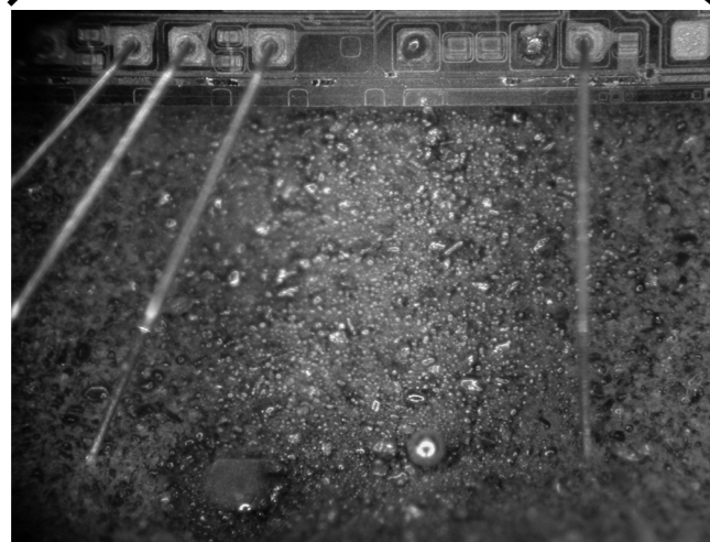
Single Event Latchup (SEL) of a high voltage driver for MEMS (vaporized bond wires)
