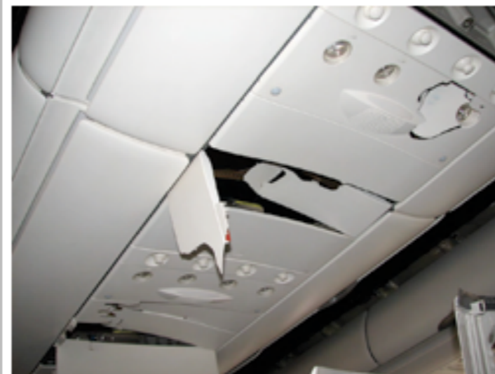
Damage from passengers collisions inside a Quantas Airbus A330 in October 2008. All potential causes for the failure of the plane's flight control system have been found unlikely, except for a radiation-induced error (SEU)
