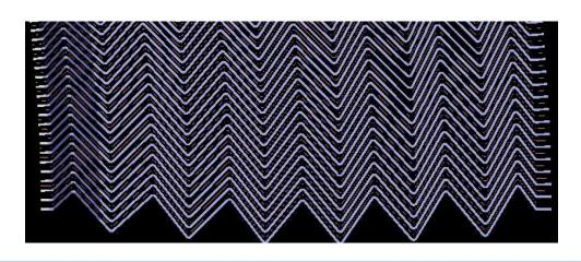
Exaggerated (10x) sagging in the EM barrel calorimeter
