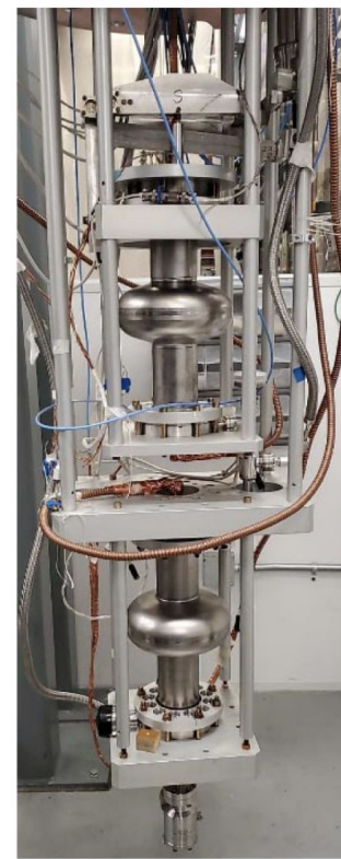
FIG. 1. Left: the experimental setup for the Dark SRF experiment consisting of two 1.3 GHz cavities. Right: a sketch of the Dark SRF electronic system.
