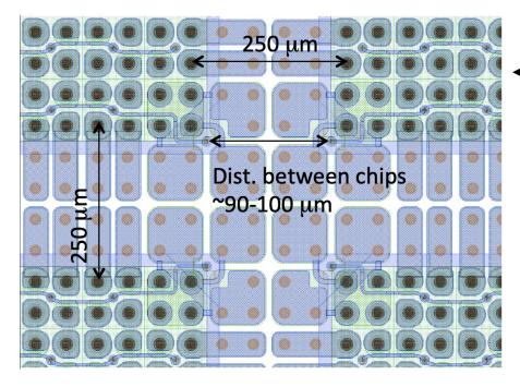
In quad modules, we expect inner-edge and outer-edge pixels to behave differently, because size of silicon pixels differ
