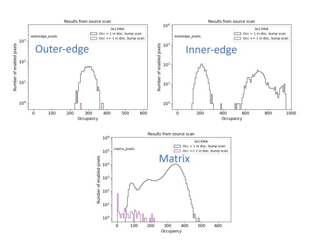
I am surprised by the difference in # of source scan counts between inner-edge pixels – is pixel sensor geometry is different in Advacam and HPK?
