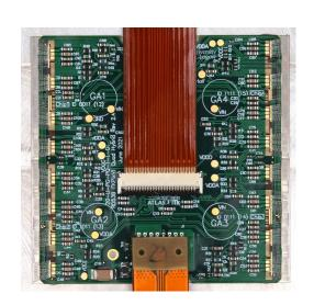
• We have 153600 pixels in each chip, and we expect chips to have less than 0.4% of disconnected bumps (600) after thermal cycling
