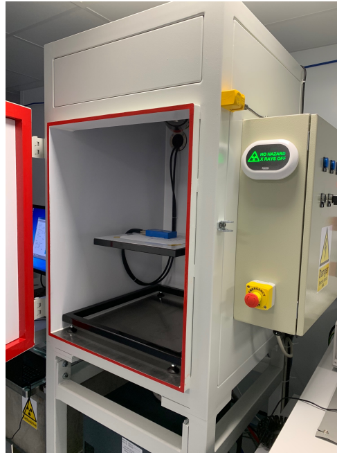
X-ray irradiation setup and beam spot @ Oxford
