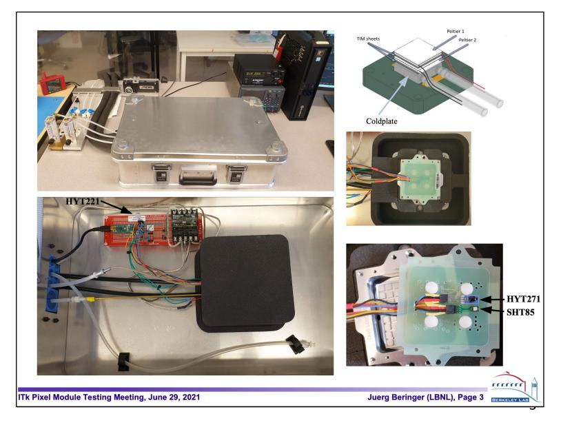
Single module cooling unit is used by most testing sites
