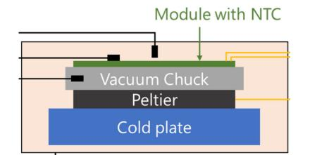
Thermal interface material between cold plate, peltiers, and vacuum chuck
