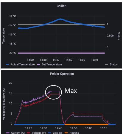
We are able to thermal cycle module from -55°C to 60°C (most extreme cycle)
