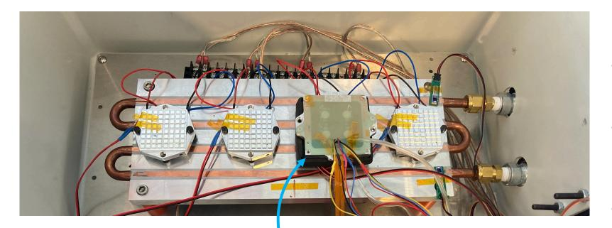
Module secured with vacuum to chuck
