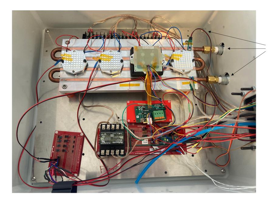
Multi-module cooling unit inside box (not thermally insulated)
