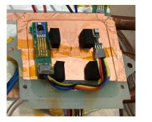
Make carrier a PCB that is in thermal contact with chuck
