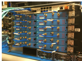
uMux readout channels (left) and NIST uMUX chip with 66 channels (right)
