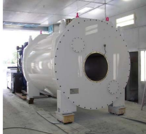
Magnet: 9.4 T, 80cm bore at University of Illinois Chicago
