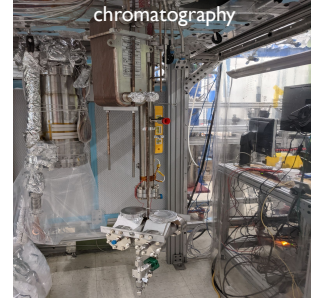
Rn suppression: Liquid Xe chromatography
