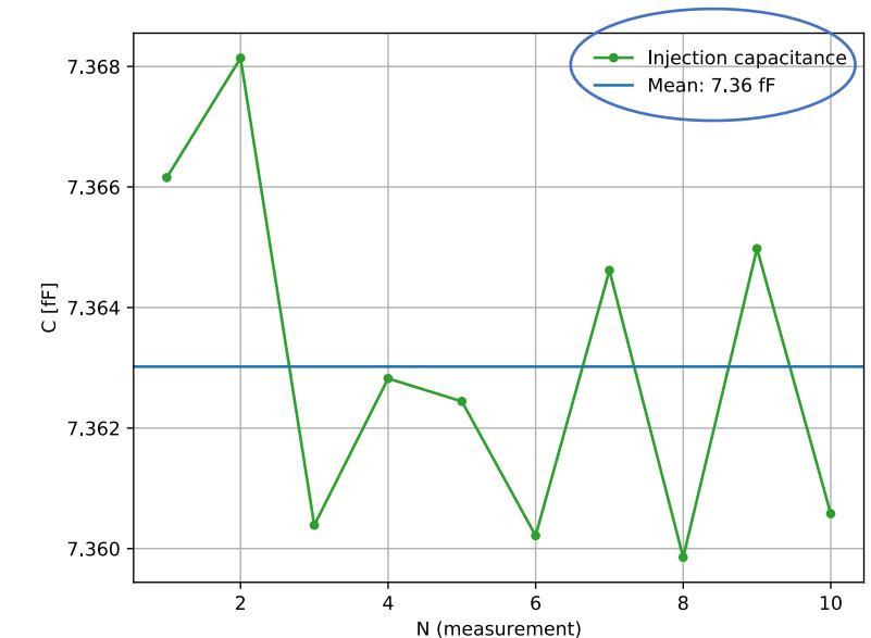
Compare average  $C_{pix}$  (7.36 fF) to nominal value (8.03 fF) → this SCC (3D, unbiased) has  $C_{pix}$  8% lower than nominal
