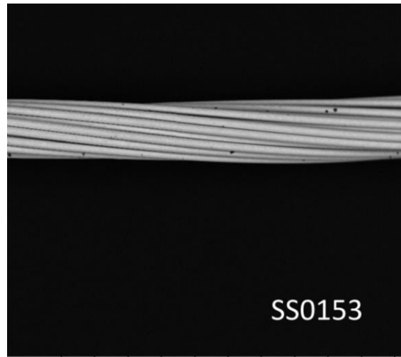
3/03/24 12:12 N D5.0 x40 2 mm 36/0.05 Strand Primary Cable (Cable Diameter: 0.33 mm)
