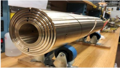
6-layer design, minimum bend radius is 30 mm
