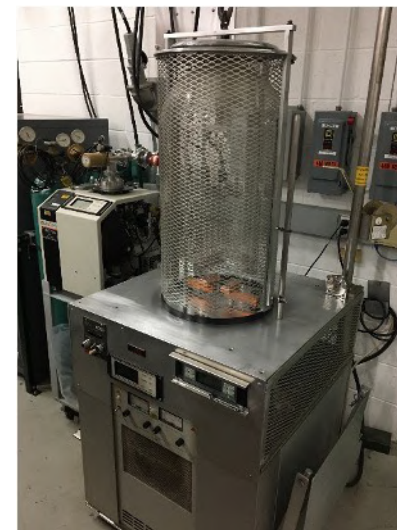
Fermilab evaporation system for CsI photocathode deposition
