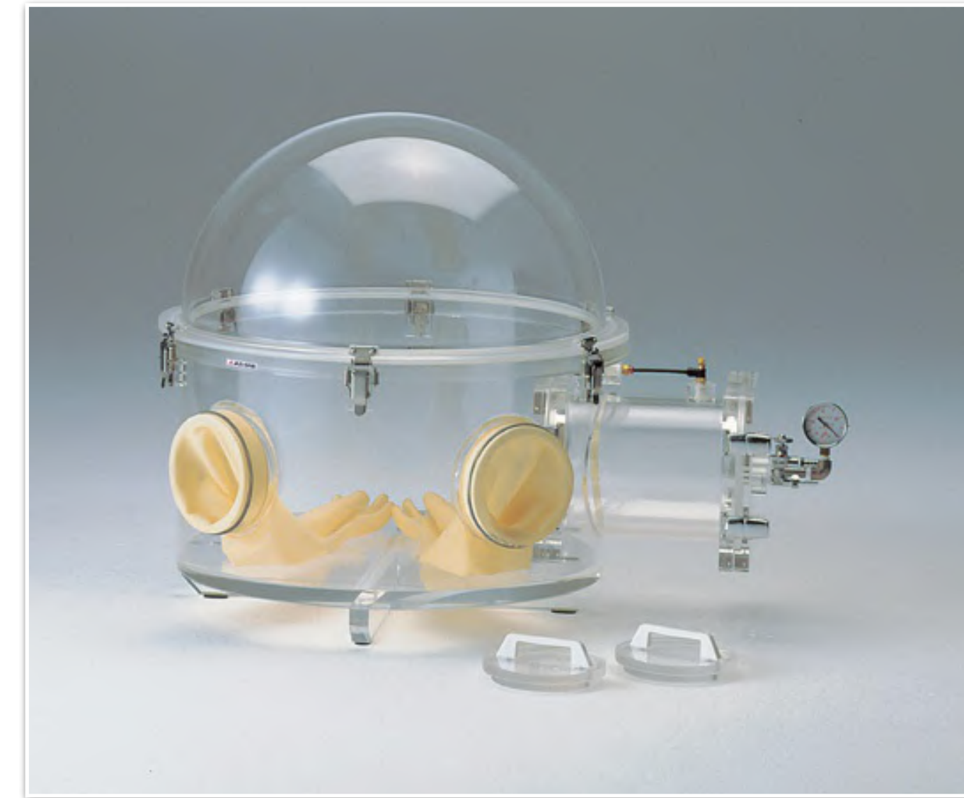
Glove box for gasPM assembly
