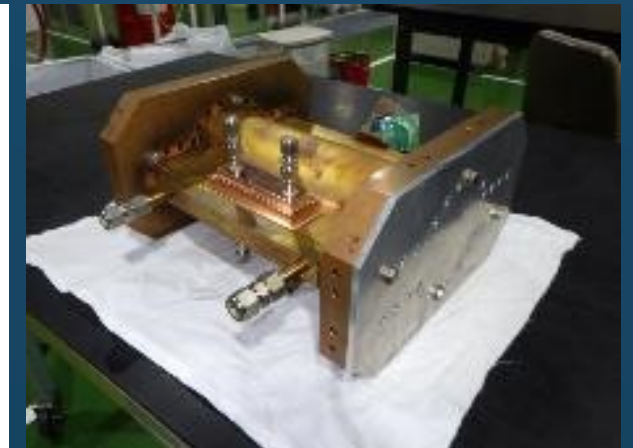
Outgassing rate measurement with prototype chamber
