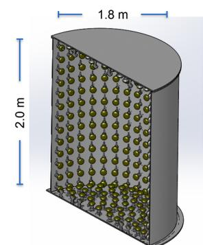
A 6-ton Water Cherenkov Detector with 3 inch photomultiplier tubes would provide excellent energy resolution and directional information for charge current interactions within a footprint feasible at First Target Station.
