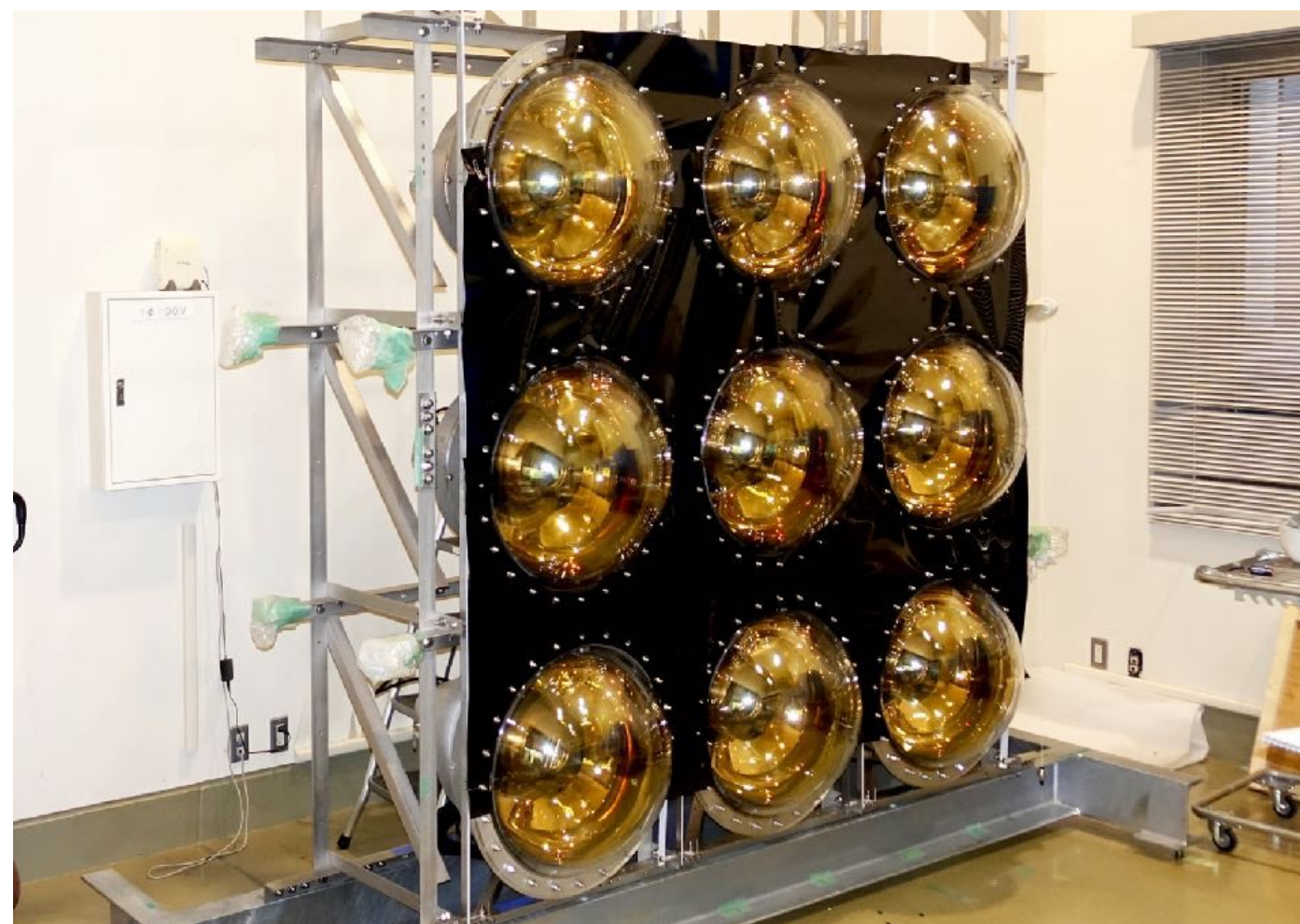
Multi-PMT module: Outer detector: PMT+WLS plate
