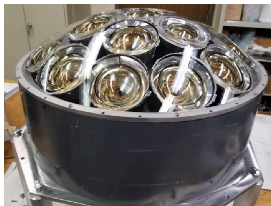
Multi-PMT module: Outer detector: PMT+WLS plate
