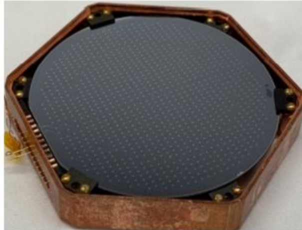
Example of a TES on silicon photon detector developed at UCB
