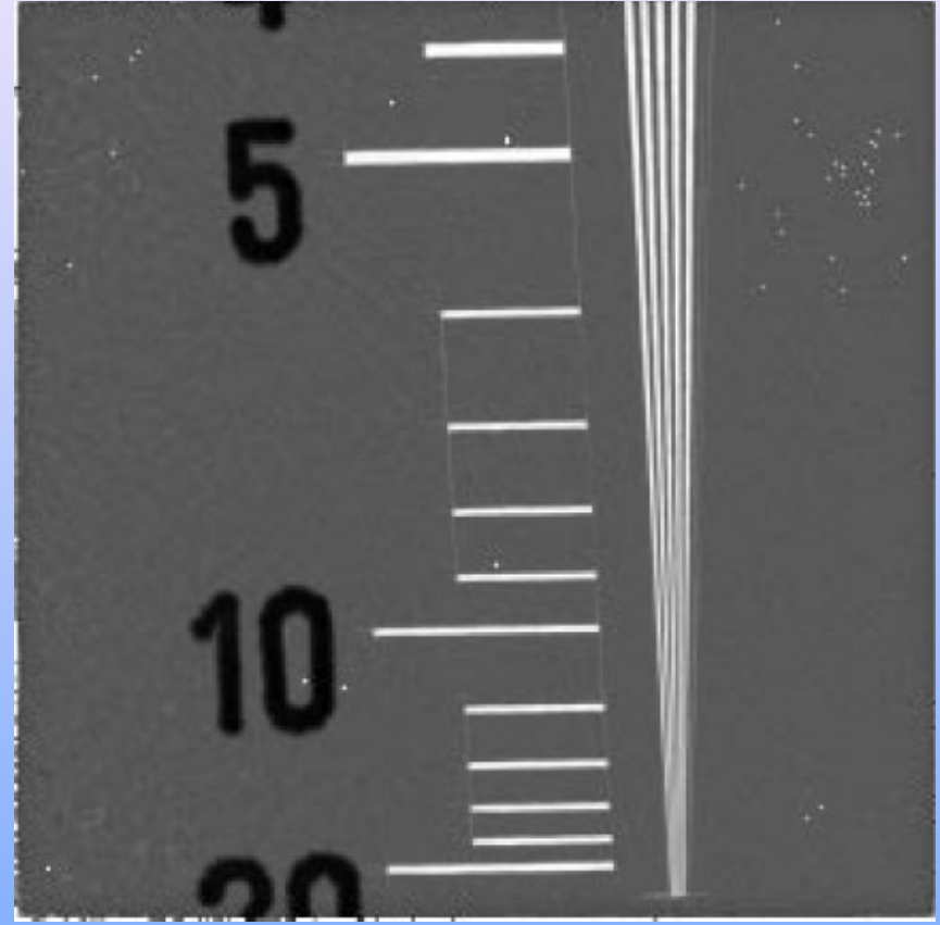
Flatfield corrected image of a lead test pattern for spatial resolution tests 1
