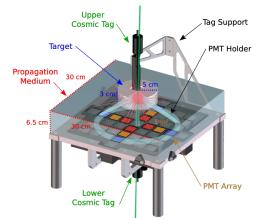
Microphysical extraction of intrinsic light yield and time profile; ring imaging; demonstration of C/S separation via timing and topology
