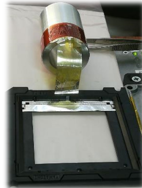
ALPIDE, SpTAB bonded to microcable
