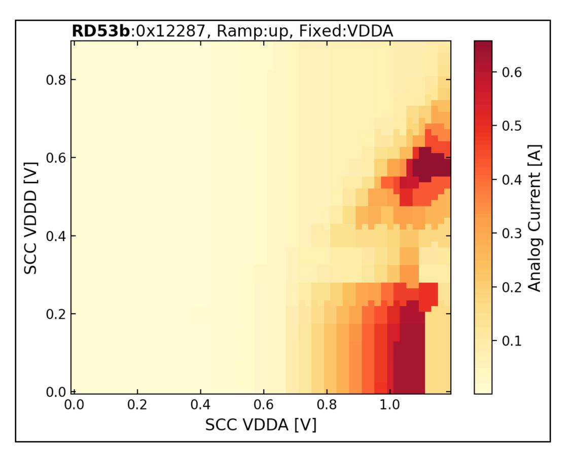
Each vertical column represents an independent scan over the quantity on the y-axis (VDDD) for the set value of the quantity on the *x*-axis (VDDA), with the specified current measurement on the *z*-axis
