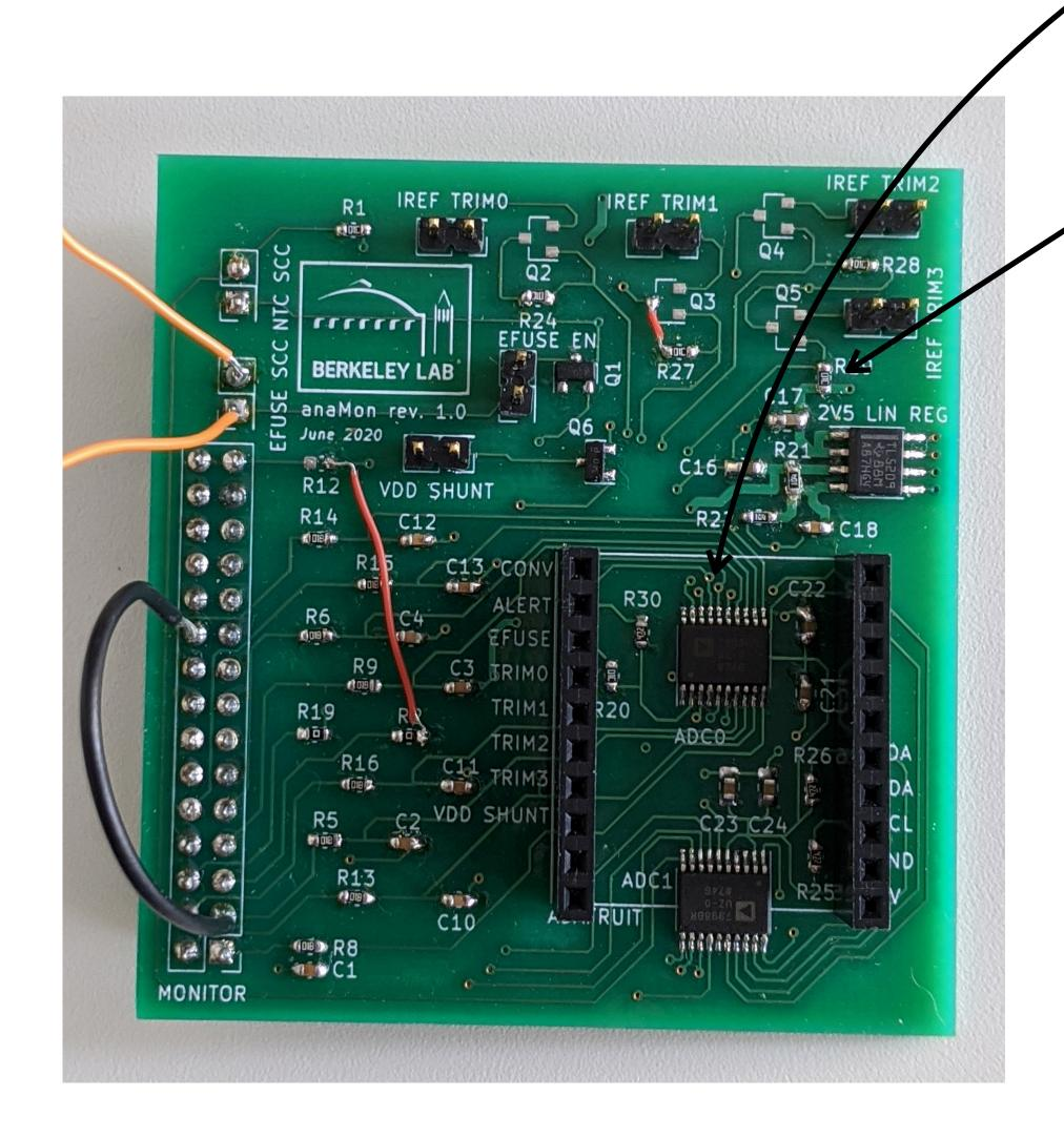
• Two on-board 8-channel 12-bit, low-power ADCs (AD7998)
