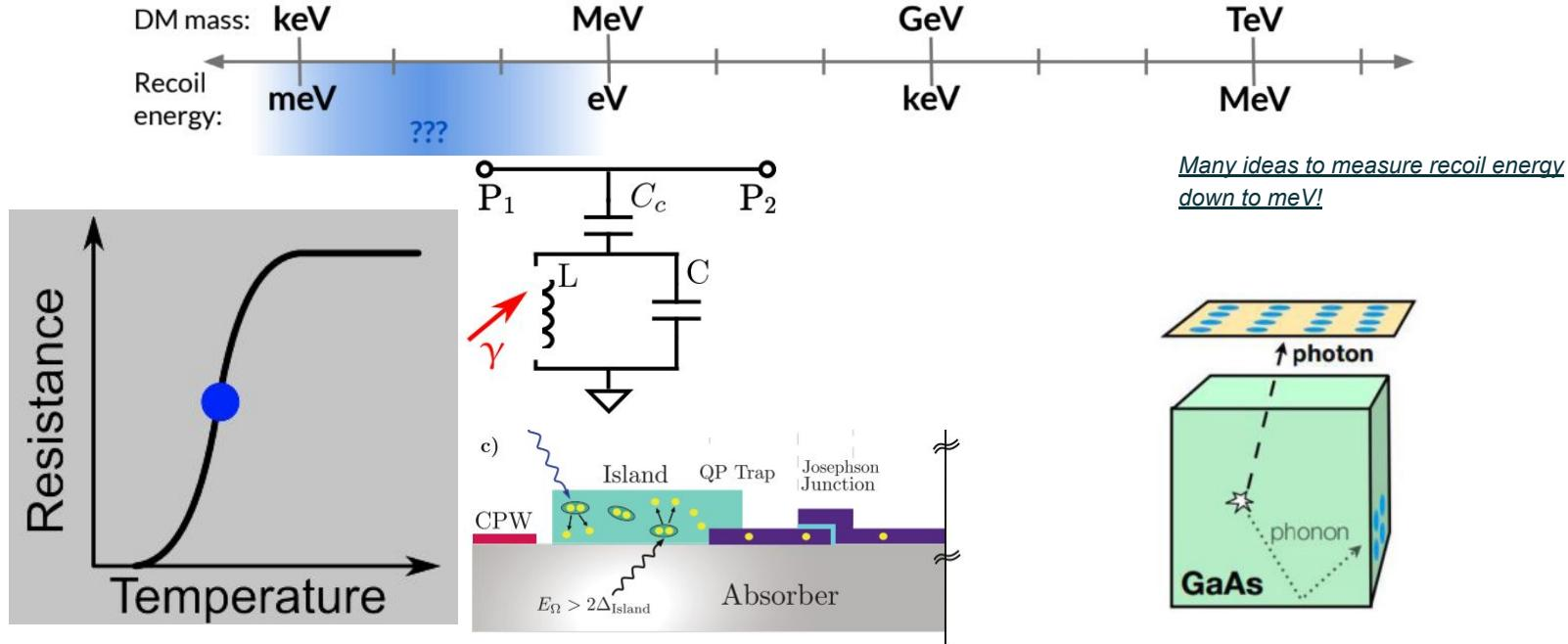
**Alternative sensors:** fundamental threshold of Cooper pair breaking energy 0.3 meV in Al
